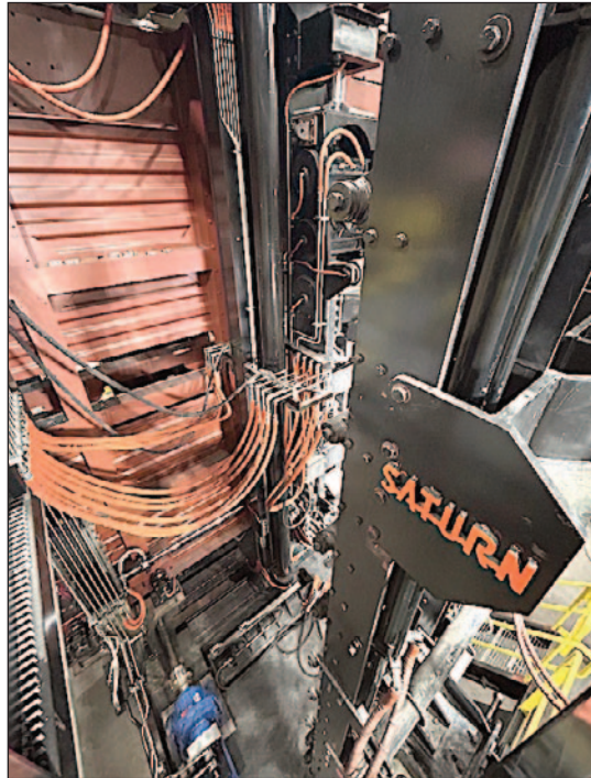
Constructed inside Saturn's 120,000-square-foot shop in Sturgis, the device at top weighs 250 tons and will be broken down in order to ship it to Pittsburgh. Pictured in the foreground are Saturn co-owners Jacob May and Charles Lynch. Directly above is May standing in the control center of the device that's the size of a locomotive and will be deployed to extract heavy doors from coke ovens for the steel-making process.
